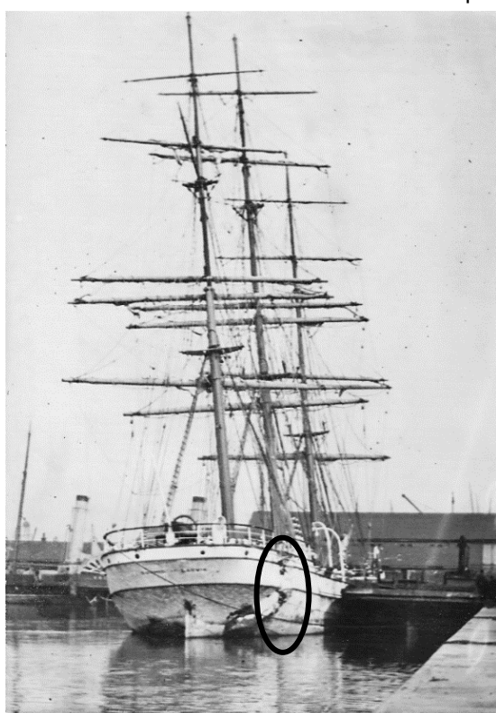
Above and right: SOPHIE under repair at Southampton and collision damage (ringed) Pictures from collection late Rod Baker
