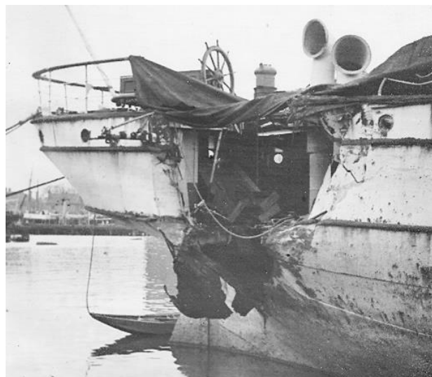
Above and right: SOPHIE under repair at Southampton and collision damage (ringed) Pictures from collection late Rod Baker
