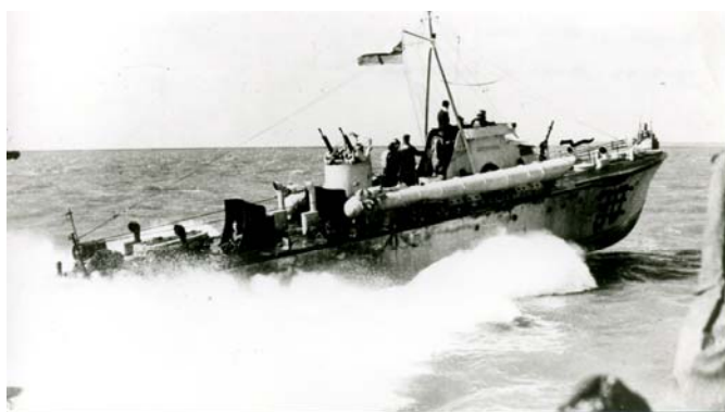
MTB 30 - Vosper 70ft design. 2-21in torpedo tubes, twin 0.5 in guns aft of bridge and single .303 abreast of bridge. This is an early boat powered by Isotta Fraschini engines
