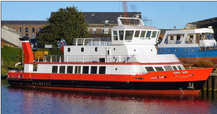
Left: Forth Hope as completed showing the remodelled bow for sea going.
